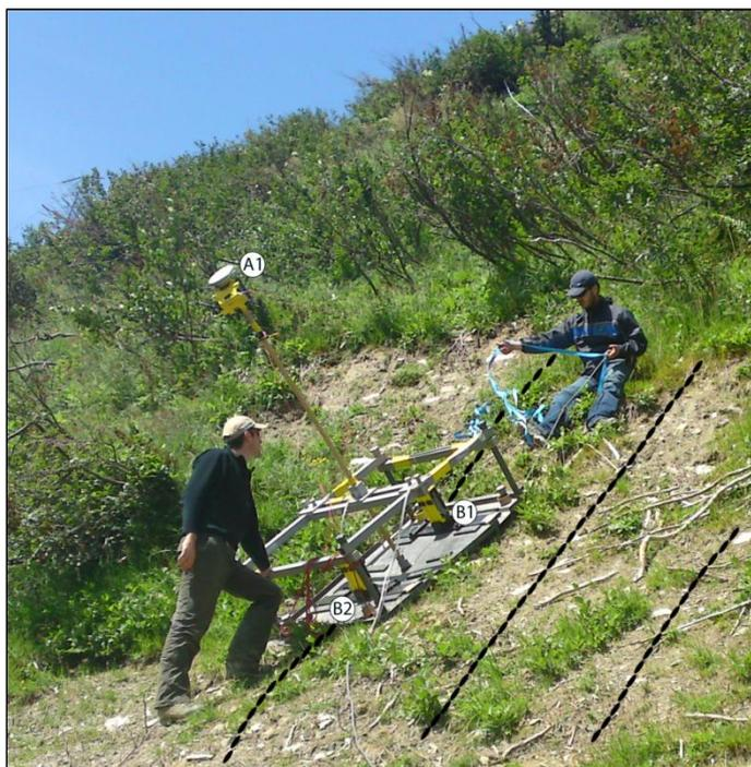
Figure 3.1: Measuring situation with the 100MHz GPR device.
