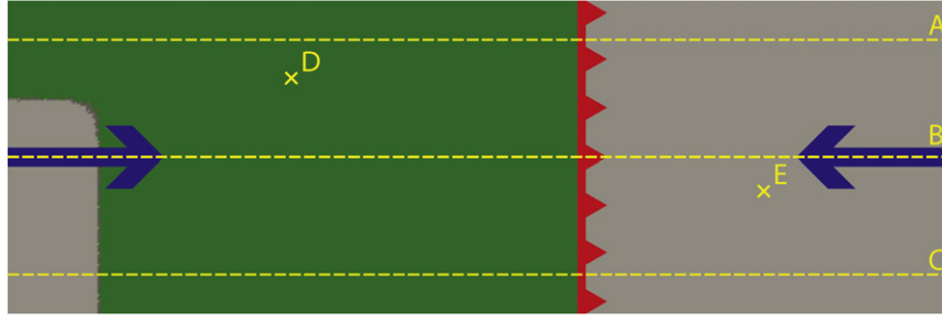
Fig. 1. Top view of the model setup used. Blue arrows indicate the direction of compression, while the red line indicates the position of the prescribed weak zone. Letters denote positions of different 2D (A)-(C) and 1D (D), (E) profiles.
